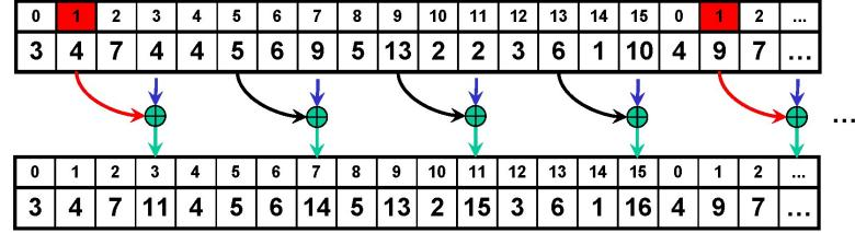
2<sup>nd</sup> iteration: 4 threads access each of 4 banks.
