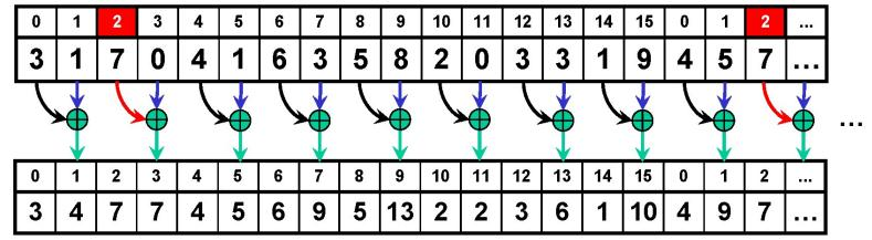
First iteration: 2 threads access each of 8 banks.
