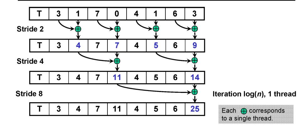
Iterate log(n) times. Each thread adds value stride / 2 elements away to its own value.
