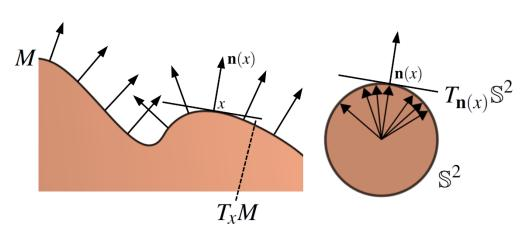
Principal curvature magnitudes and directions are eigenvalues and eigenvectors of shape operator **S**
