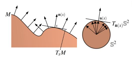
Principal curvature magnitudes and directions are eigenvalues and eigenvectors of shape operator **S**
