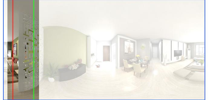
Fig. 4: **Panoramic slice** One of the slices produced by the network, placed at its position within the equirectangular image. The red line shows the area sampled by the right eye, while the green line shows the area sampled by the left eye (see Fig. 2b). In the background, we see the original panorama from the central viewpoint (note the large shift due to parallax effects).
