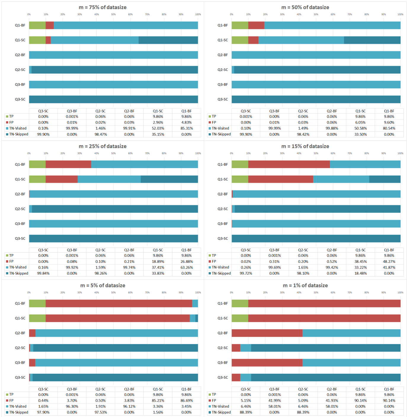
Fig. 15. Visualization of the statistics given in Table 6 for the Synthetic Perlin Noise data set. True positives (TP) are shown in green, false positives (FP) in red, and true negatives (TN) in blue. BF denotes Bloom filters without supercells, and SC with supercells, respectively. For the stacked bar charts using supercells (SC) the two shades of blue denote TN not skipped by hierarchical supercell early-out (lighter blue) and TN skipped by hierarchical supercell early-out (darker blue), respectively. The latter is denoted by SC-Skip in Table 6.
