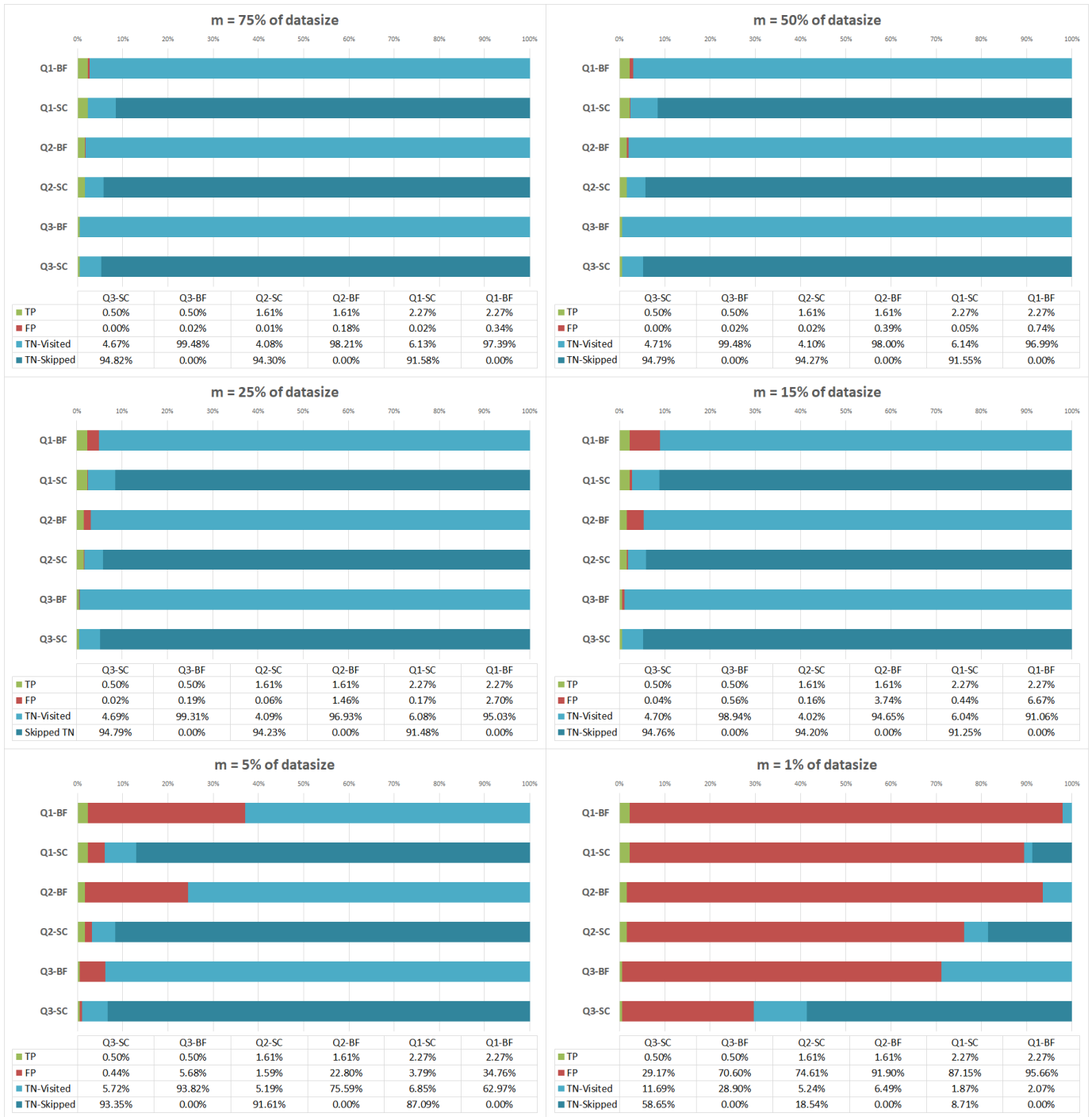
Fig. 14. Visualization of the statistics given in Table 6 for the Red Sea data set. True positives (TP) are shown in green, false positives (FP) in red, and true negatives (TN) in blue. BF denotes Bloom filters without supercells, and SC with supercells, respectively. For the stacked barcharts using supercells (SC) the two shades of blue denote TN not skipped by hierarchical supercell early-out (lighter blue) and TN skipped by hierarchical supercell early-out (darker blue), respectively. The latter is denoted by SC-Skip in Table 6.
