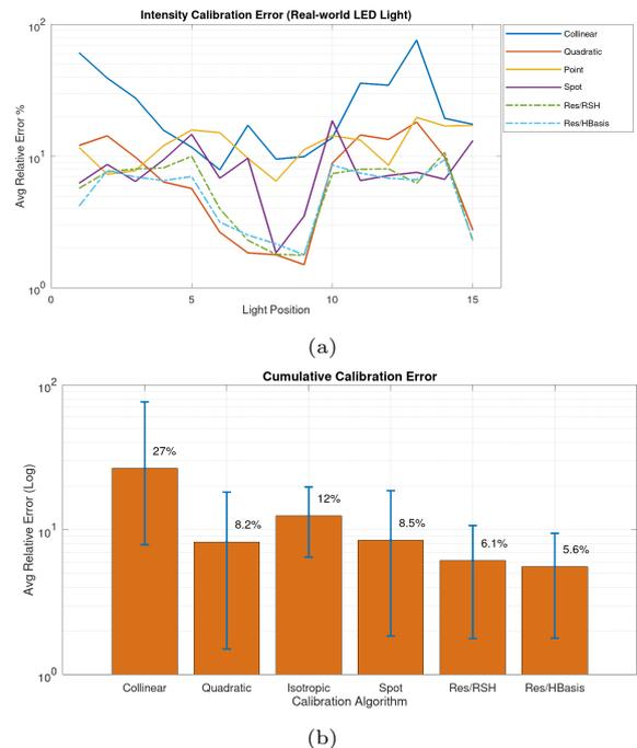
Fig. 7: Non-centered light axis. Average relative error values computed (a) for each image, and (b) across all MLIC images and all light types. Vertical lines are minimum/maximum errors. *Quadratic* and *Spot* exhibit an error up to 20%, and up to five times bigger than the proposed approach. *ResidualRSH* and *ResidualHBasis* prove to be more stable/reliable across different lighting conditions.
