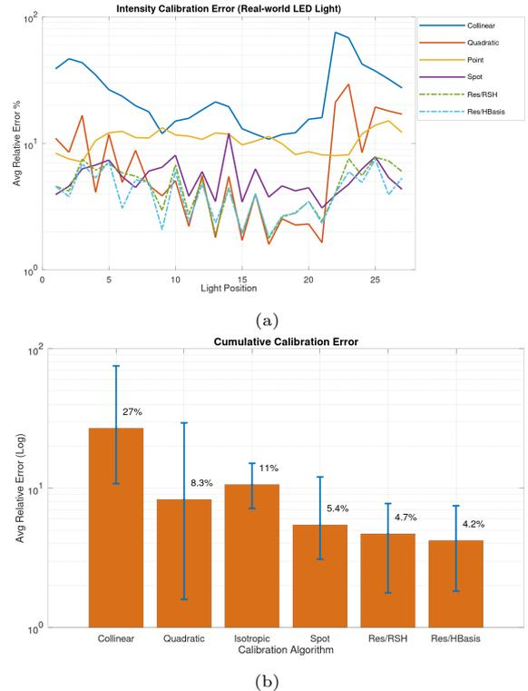
Fig. 5: Spectralon MLIC. Average relative error values computed (a) for each image, and (b) across all MLIC images and all light types. Vertical lines are minimum/maximum errors. *ResidualRSH* and *ResidualHBasis* prove to be more stable/reliable across different lighting conditions.
