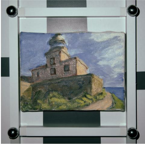
Fig. 1: MLIC acquisition setup. The camera points toward the object, surrounded by some calibration targets (glossy spheres and a white frame).
